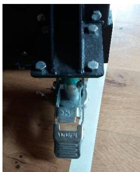
These are located at the rear of the unit on each side fixed to the two rear columns. When the whole structure is to be moved into a new location put these in the **up** position, with the rubber pads clear of the flooring, by pressing the 'up' lever.
