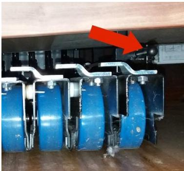
Before extending the seating the 2 row locks must be released. They are the 2 **outer** black knobs located on each side of the seating unit, adjacent to the cluster of blue wheels, indicated by the arrow in the picture. Release them both by pushing on them while gently pulling on the pulling handles.
