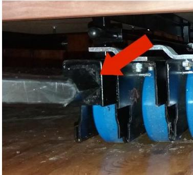
The telescopic platforms must be opened by two persons working together. Insert the two T-shaped pulling handles into the front of the row 1 columns. The pulling handle is entered at an angle of 30° from the horizontal and when inserted fully twisted to the upright position. The handle is now locked into the correct position for pushing and pulling. **Keep hold of the handle when it is in the upright position so it does not fall and dent the floor.**
